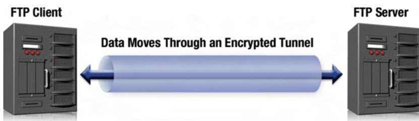
One of the main differences between SFTP and FTPS is the way authentication is performed. With SFTP, clients can be authenticated with just a password or a Private Key. With FTPS, clients and servers can be authenticated with certificates, which are either self-signed (by your organization) or signed by a Certificate Authority (e.g. Verisign).
